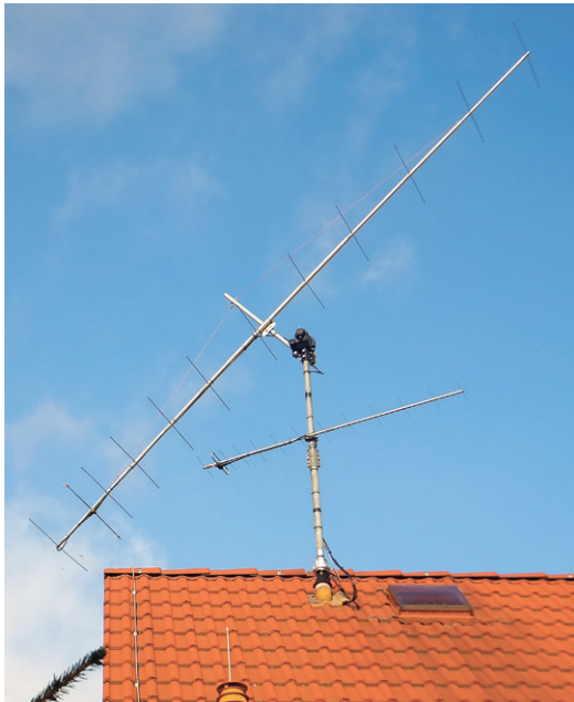
Figure 5 — The 12-element Yagi antenna used by DL1VPL to complete DXCC on 144 MHz. [Thomas Hartig, DL1VPL, photo]
