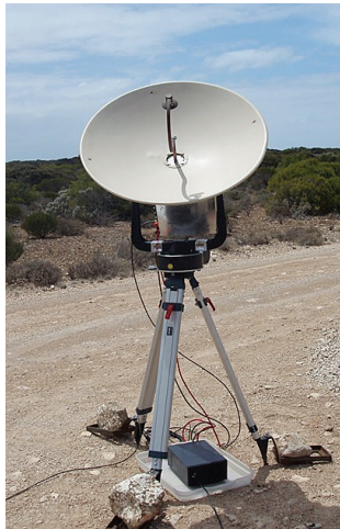
Figure 6 — The portable EME-capable 10 GHz station of VK7MO, set up at roadside in the Australian Outback. [Rex Moncur, VK7MO, photo]
