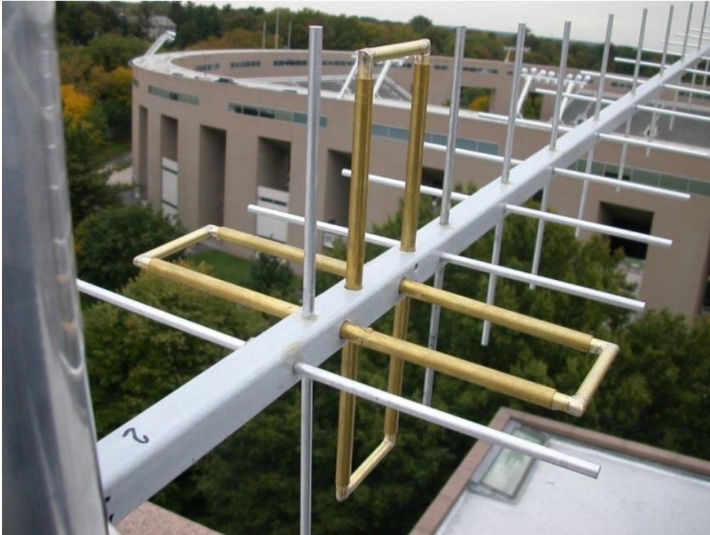
Fig. 5. – Rear view of a single LFA15-JT Yagi showing construction details around the driven elements. The brass loops are fed at the split centers of their forward sides, inside the hollow boom. RG142 coaxial feedlines pass out to the rear. All elements are held in place with tight-fitting holes and a few drops of fiberglass resin.
